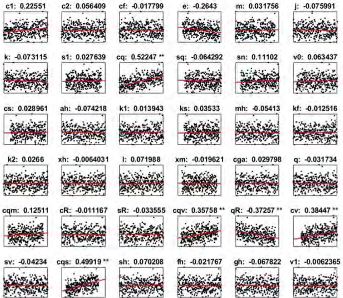
Figure 5.5: Using a Latin Hypercube, 360 randomized parameter combinations were generated within the parameter value \pm 10\% . The values for the parameters were plotted on the x-axes and the tumor's ultimate growth rate was plotted on the y-axis. Correlation coefficients were determined for each pairing of parameter and the tumor growth rate; the parameter and correlation coefficient are listed above each subplot. Any parameter with correlation greater than the arbitrary value of 0.3 is marked with two asterisks.
