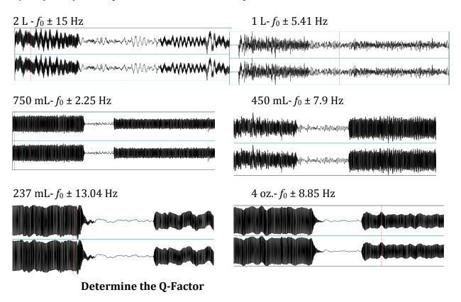
Using the data from above and the formula,  $Q = f_0/\Delta f$ , we determined the Q-factor for each bottle.
