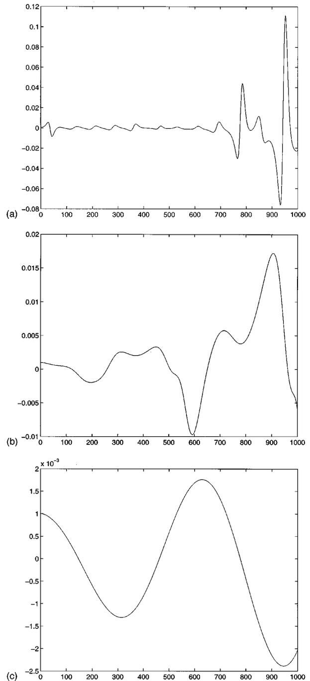
FIG. 9. The difference in  $x$ -values (vertical axis) between chaotic trajectories with reference IC (1,1,1) and new IC (0.999, 1, 1) vs. 1000 time steps of the integration (horizontal axis) for (a) Eqs. (1)–(3), (b) Eqs. (6)–(8), and (c) Eqs. (9)–(11). For all trajectories, the integrations are sampled every step with  $h=0.01$ . All computations are double precision with  $x$ -values rounded to six decimal places.
