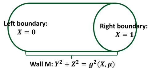
Figure 1: Schematic illustration of our ion channel modeled by  $\Omega_\mu = \{(x, y, z): 0 < x < 1, y^2 + z^2 < g^2(x, \mu)\}$ , where  $g$  is a smooth function satisfying  $g(x, 0) = 0$  and  $g_0(x) = \frac{\partial g}{\partial \mu}(x, 0) > 0$  for  $x \in [0, 1]$ . The boundary consists of three portions, where the left and right boundaries are viewed as the ends and M is considered the wall of the channel.
