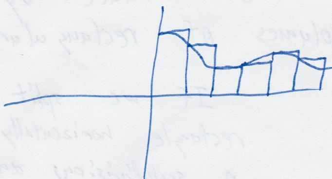
$f(x) \geq 0$ , we used a Riemann sum to estimate the area under the curve of  $f$ :
