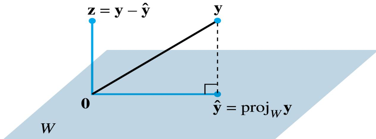
The orthogonal projection of  $\mathbf{y}$  onto  $W$ .
