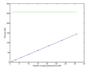
Figure 3: Graph of File size vs. Number of values preserved out of 64. The original file size is plotted in green above
