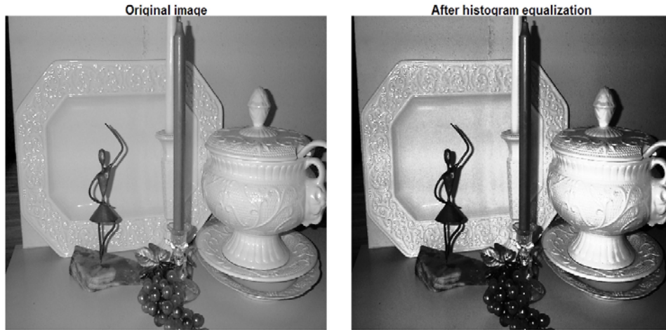
FIGURE 12.7. Two images produced by function histgr . Histogram equalization is done by commercial software. Use your own histogram equalization image processing technique to see if the result is the same.
