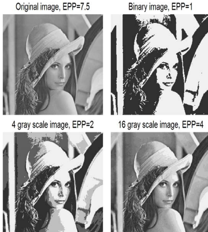
FIGURE 12.5. The original image Lena, the canon of image processing, and three optimal reductions with minimum information loss. The Entropy Per Pixel (EPP) of the original image is close to the absolute maximum, 8 bits. Information in the binary image is almost one-eighth of that in the original image.
