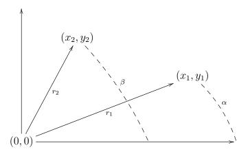
Let  $\theta$  be the angle between the vector  $\vec{v_1}$  from (0,0) to  $(x_1, y_1)$  and the vector  $v_2$  from (0,0) to  $(x_2, y_2)$ . Express the cosine of  $\theta$  in terms of  $x_1, x_2, y_1, y_2, r_1$  (the length of  $\vec{v_1}$ ), and  $r_2$  (the length of  $\vec{v_2}$ ).
