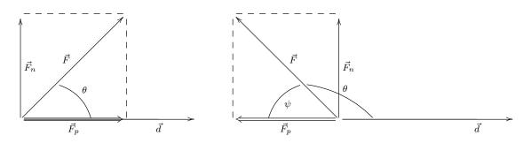
If  $\vec{F}$  makes an angle of  $\theta$  with  $\vec{d}$ , then the component of  $\vec{F}$  along  $\vec{d}$  is
