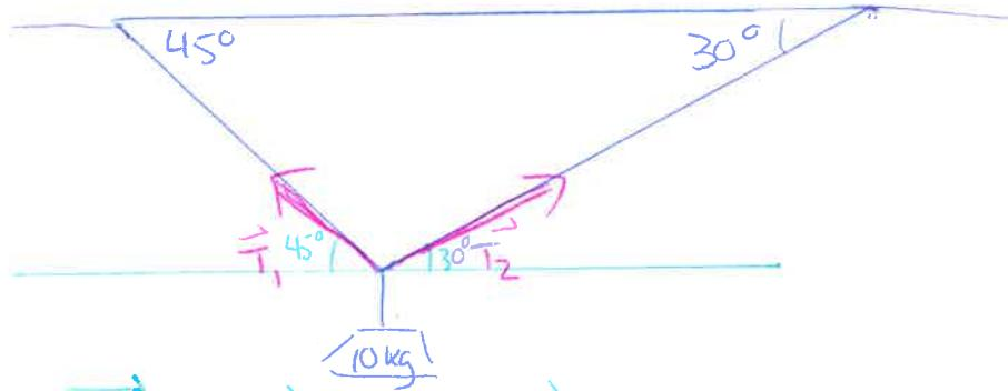
We know that  $\vec{T}_1 + \vec{T}_2 = -\vec{F}_g$ , where  $\vec{F}_g$  is the force caused by the gravity.
