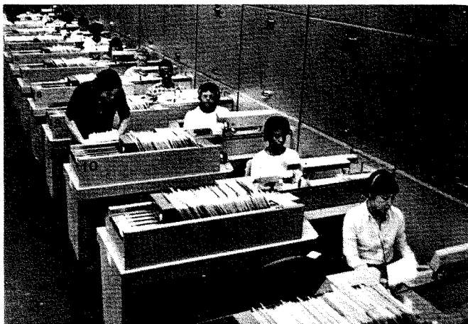
Fig. 29 Multi-Position Letter Sorting Machine
