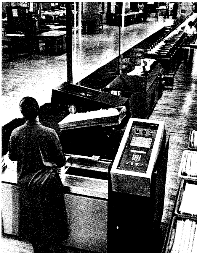
Fig. 28 Optical Character Reader/Channel Sorter
