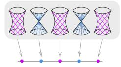
Most fibers will be smooth quadric surfaces, which have two rulings of lines. Finitely many of the fibers will degenerate to singular quadrics, and assuming only simply degeneration, they will have just one ruling of lines (simple degeneration will follow automatically if the quadric surface fibration comes from a pencil of quadrics containing a smooth complete intersection; see [Rei72, Proposition 2.1]).
